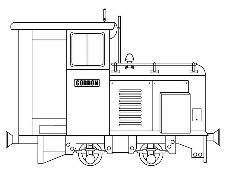
Built in 1978 for the National Coal Board Gordonwas a flame proof locomotive for working in and around mines. Working at Allerton Bywater and Castlebridge mines the loco is fitted with a Perkins engine, thatwas built in Stafford. After her working life she ended up in a scrap yard in Fife, from where she was purchased. Arriving at Amerton in 1996.
