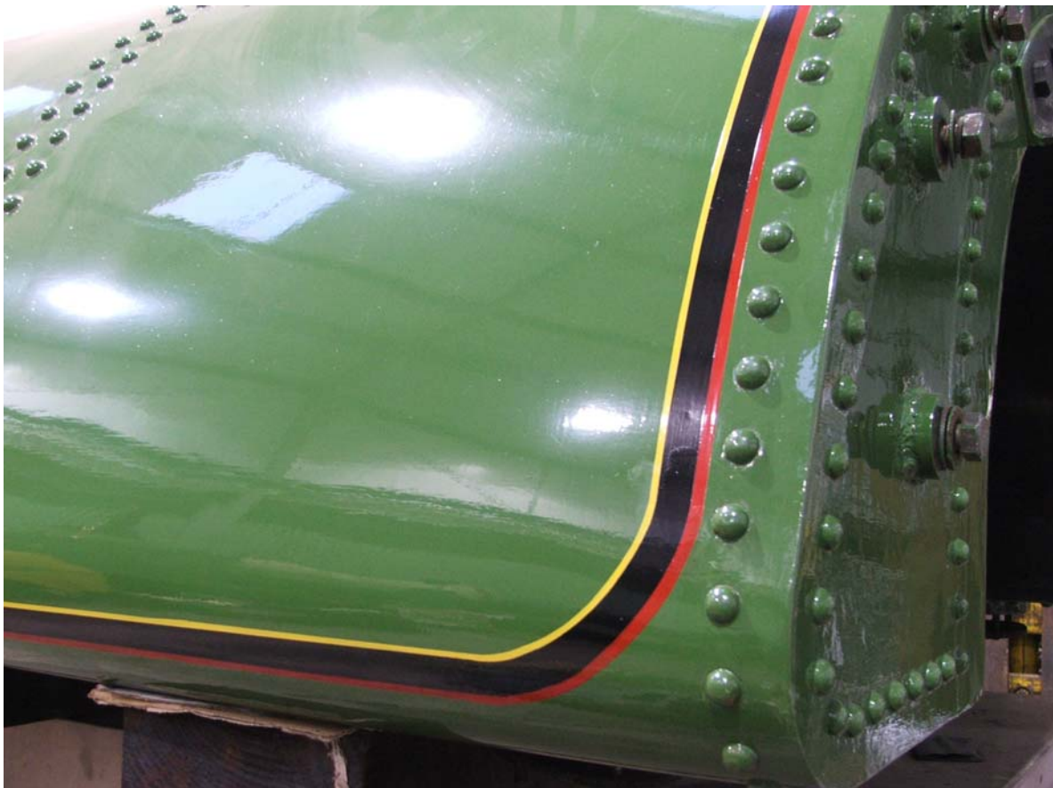
The new Bagnall lining seen here on Isabel's saddle tank – a very fine job indeed.
