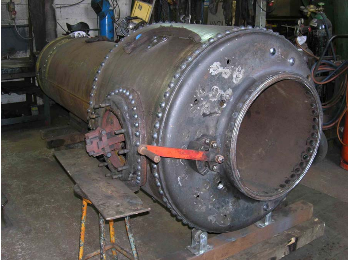
Isabel's boiler nearing completion in Derbyshire, note the regulator valve
