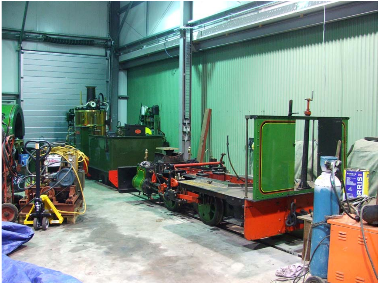
Isabel sits in the workshop, boiler removed
