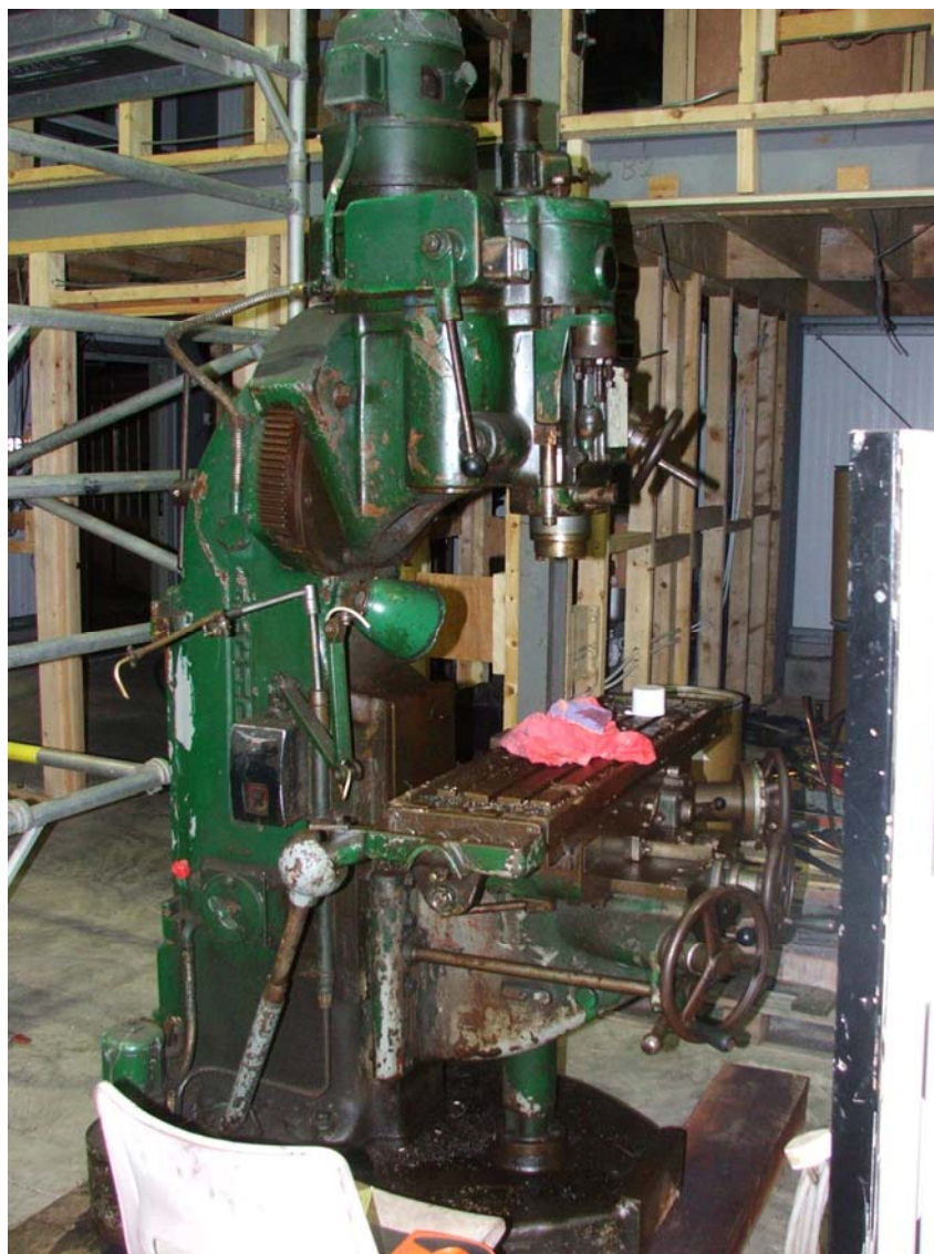
The 1940's Archdale milling machine, ready to be installed in the machine shop.
