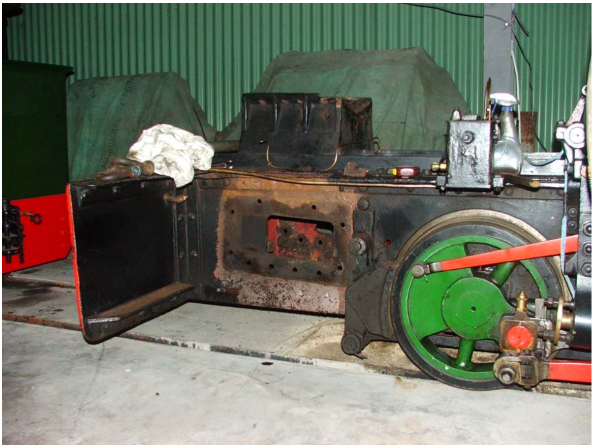
The cylinders removed from Isabel, note the area of wasting near the frame angle
